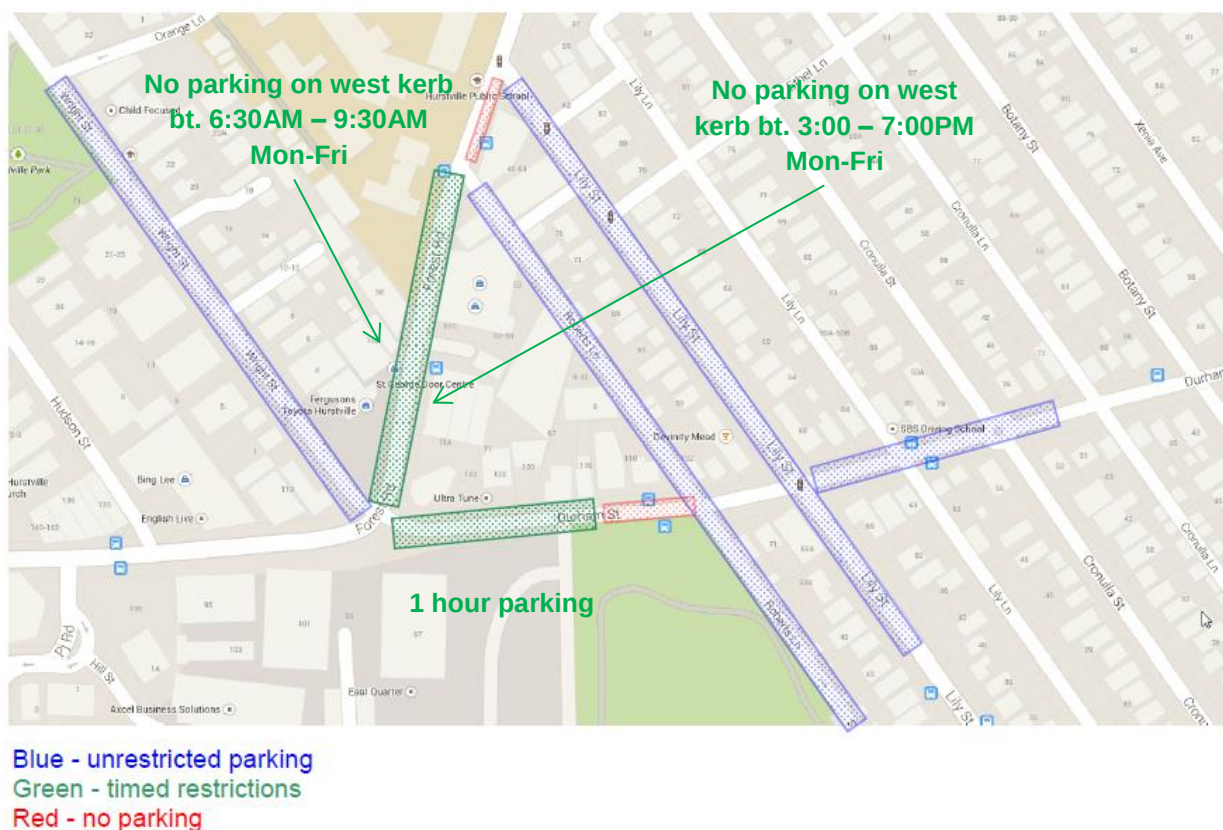
Figure 3.6: Existing on-street car parking controls
